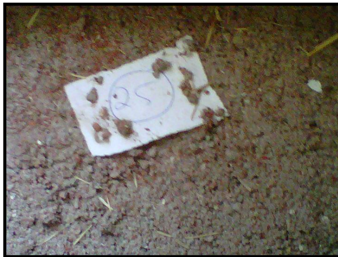
Figure 4.6: insufficient cement in the mix
