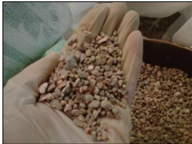
Figure 3.18: particles passing sieve (No. \frac{1}{2} ) and retained on sieve (No. \frac{3}{8} )
