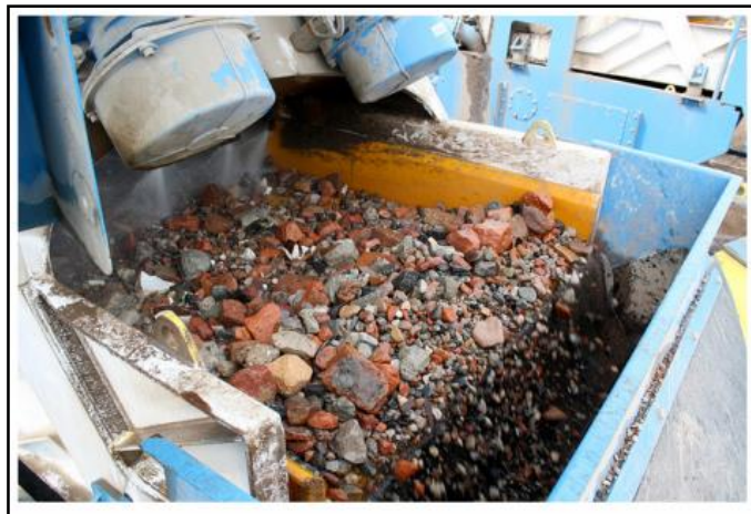
Figure 3.12: Washing recycled aggregates (Craven, 2009)
