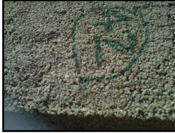
Figure 4.9: Lack of Fine particles/high porosity
