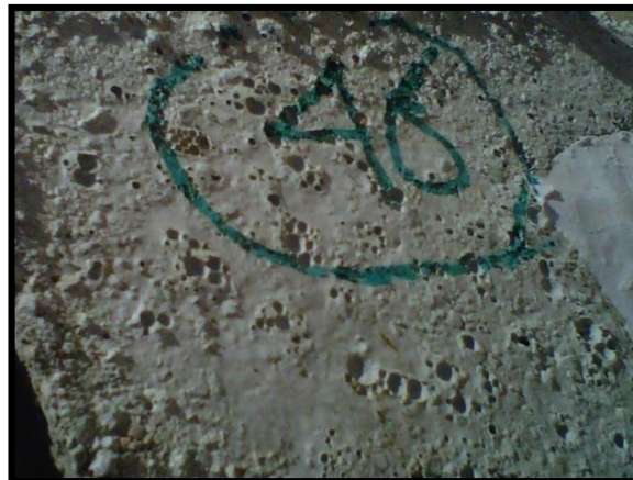
Figure 4.8: Bubbles resulting from water
