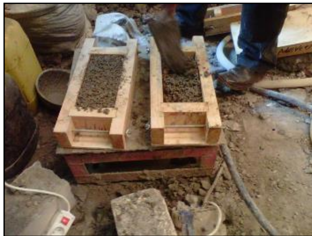
Figure 3.22: Placing molds on the vibrator
